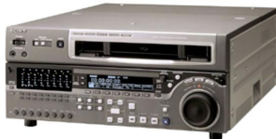
And there is the **HDW-M2000/1** [US\$ 60,000] which can play and record 1080/59.94i, 50i, 29.97PsF, and 25 PsF. It can also play back [but not record] tapes at 24PsF and 23.98 PsF. Incidentally, this VCR can play back Betacam and Digital Betacam tapes as well, and convert them to 1080i for use in an HD production.
